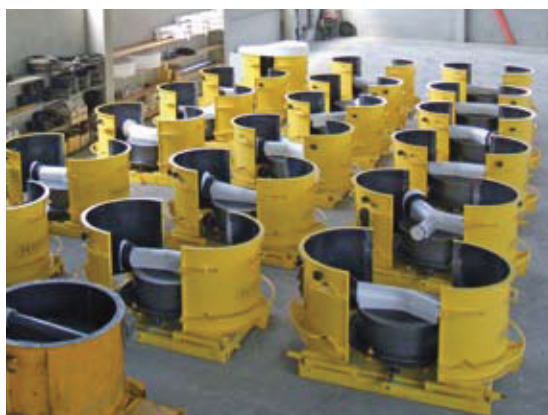
Fig. 2b Prepared with form parts made of polystyrene the molds are ready now for casting.
