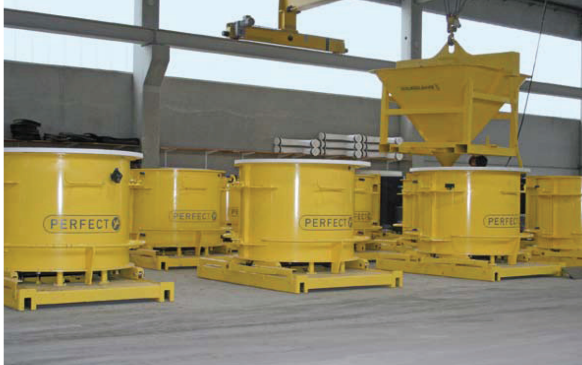
Fig. 2 a 18 molds for the production of manhole bases at Josef Heller & Sohn are positioned in a stationary arrangement in the curing area.
